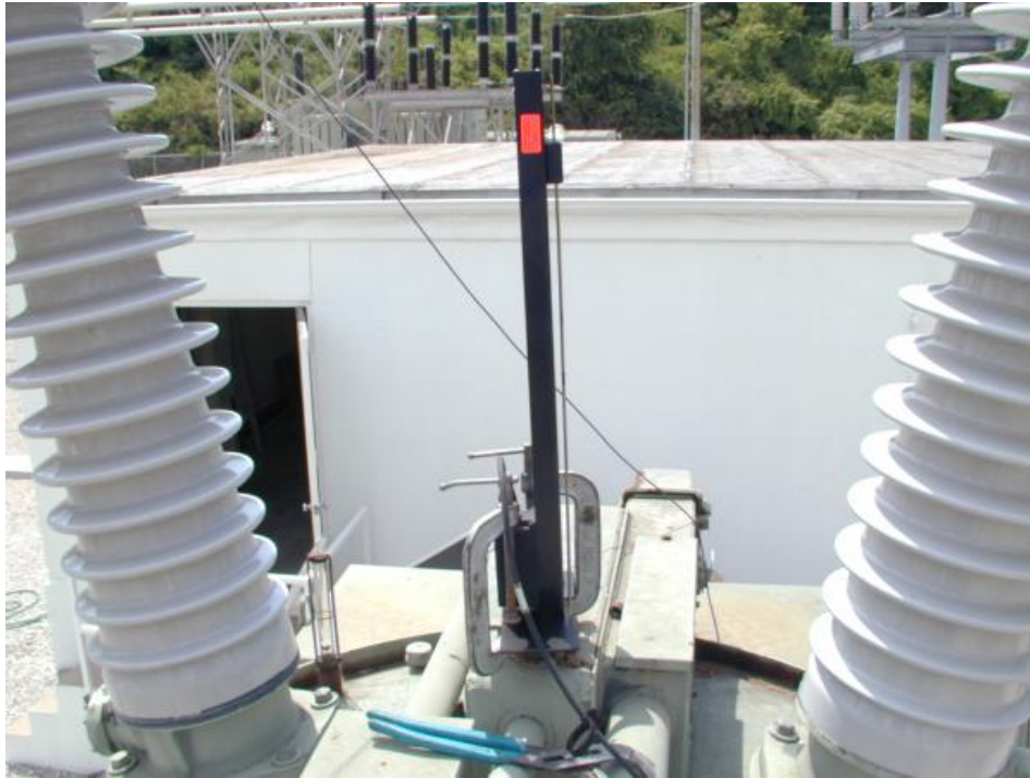
Linear Transducer on an OCB
